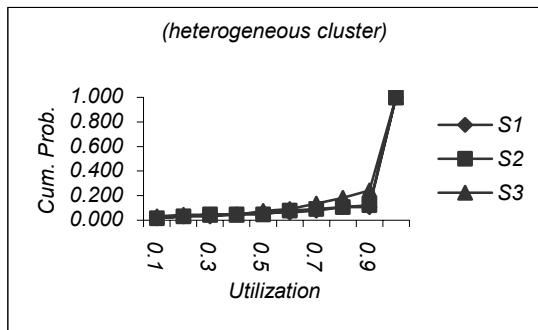
**Figure 7: Probability of saturation of servers using LU**
