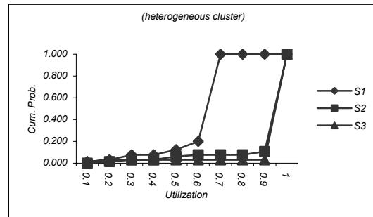
**Figure 6: Probability of saturation of servers using RR**
