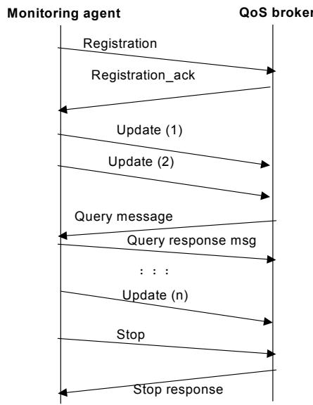
**Figure 4: Protocol between monitoring agents and the broker**
